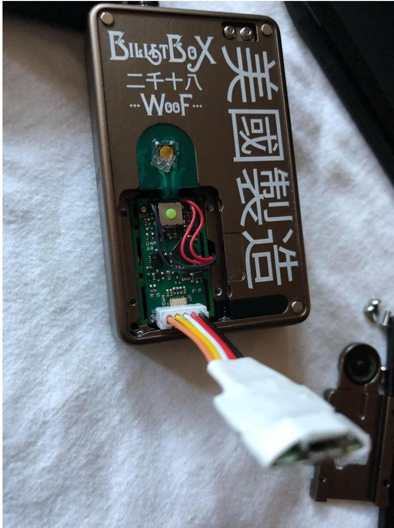
9.) Once the BS is seating clearly in the DNA, using one hand pinch the USB end of the BS then using your other hand, plug your connected micro USB cable into the DNA60 USB board.
