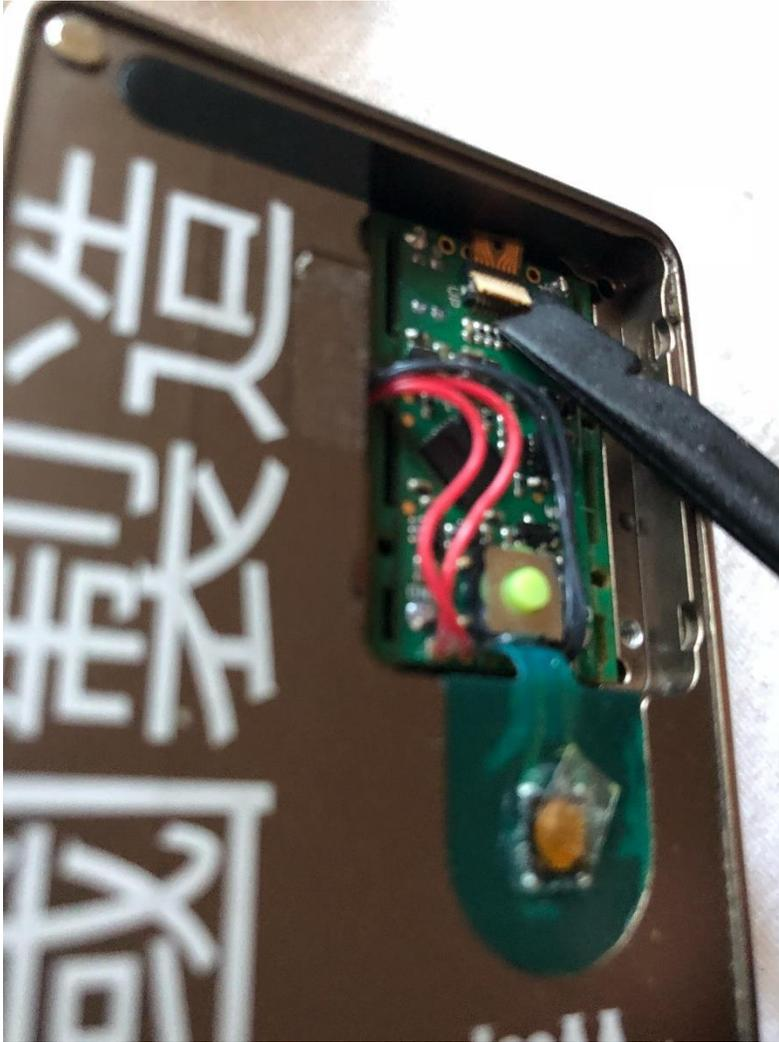
7.) Using the pointed end of spudger tool, locate the small hole in the screen cable, insert the tool and slowly remove screen from connector.
